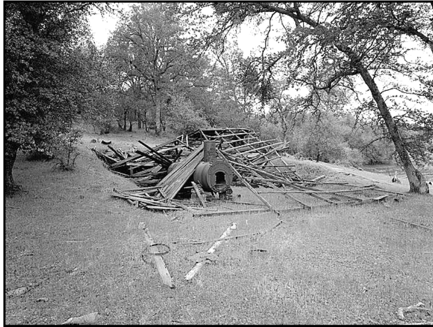
Figure 51: Tractor-boiler that Supplied Power to Two-stamp Mill at Defiance Claim (Library of Congress, HAER Photo by Alice Olmstead).
